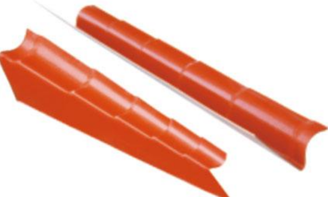
NSME:LEFT/RIGHT SIDE GABLE FLASHING EFFECTIVE LENGTH: 1090 MM WIDTH: 150 MM × 98 MM PURPOSE:GABLE SIDE FLASHING GUIDES WATER OFF THE ROOF.
