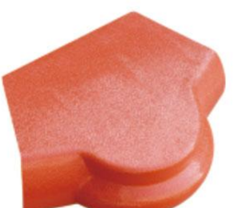
NSME:RIDGE CAP END SPECIFICATION:LENGTH: 300 WIDTH: 90 HIGH: 220 PURPOSE:USED TO COVER THE END OF THE MAIN ROOF RIDGE.
